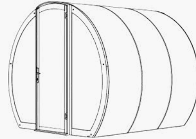
6 Person Meeting Pod L2420mm x W2500mm x H2100mm Structure = 370kg Table = 48kg LED lighting = 2kg
